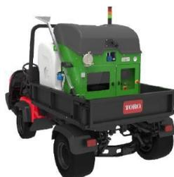
Small capacity Foamstream mounted on a utility vehicle
